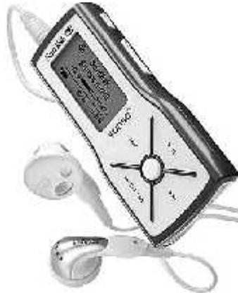
The picture to the left is a ScanDisk MP3 Player similar to the one that the author uses for portable operation. I use it to send CQ on SSB and record QSOs . It measures only 3" x 1.25" x 1" and weighs-in at about 2 ounces!
